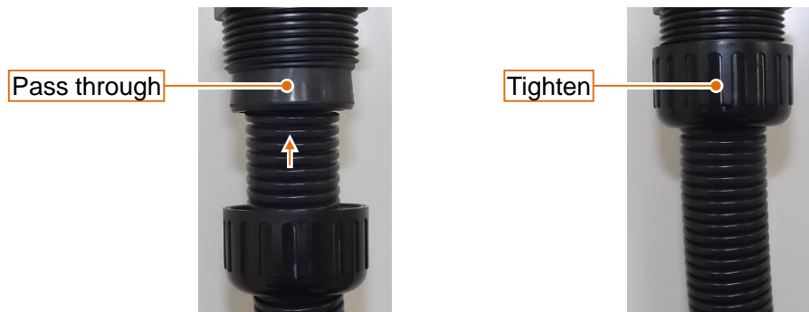
Fig. 40 Tightening the sealing nut
